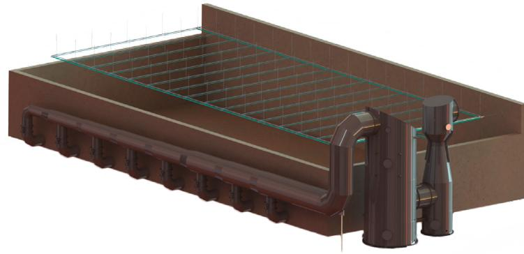
This system ensures permanent filter humidification to guarantee optimal conditions for the growth and distribution of flora, because the effectiveness of a biofiltration system is strongly dependent on the water content of fillers and relative humidity.
